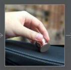
5.Paste in the flat position (With the pressure of not less than 3 kgs and lasts more than 10 seconds, then use it 24 hours later
